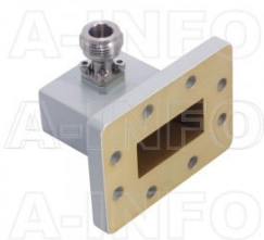
137WCAN Right Angle Rectangular Waveguide to Coaxial Adapter 5.85-8.2GHz WR137 to N Type Female
