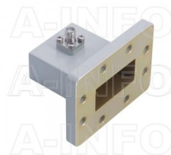
137WCAS Right Angle Rectangular Waveguide to Coaxial Adapter 5.85-8.2GHz WR137 to SMA Female
