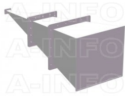
LB-137-25-ASPO Standard Gain Horn Antenna 5.85-8.2GHz 25dB Gain Rectangular Waveguide Interface
